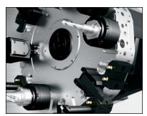
Both DS machines are equipped with a hybrid turret that accepts BOT tools, OD tools and VDI 40 tools. The DS-30Y has a 12-station turret, and the DS-30SSY has a 24-station turret.
