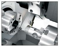
Dual-spindle turning combined with Y axis, C axis, and high-torque live tooling allow multiple operations in a single setup to reduce part handling and increase accuracy.
