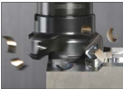
The Haas 50-taper spindle features a 30 hp vector drive system that provides 450 ft-lb of torque for heavy cuts.
