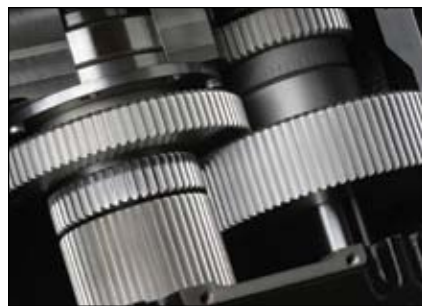
The Haas-built two-speed gearbox provides a versatile combination of high torque in low gear and speeds to 7500 rpm in high gear for added flexibility. The gearbox is isolated by polyurethane mounts to eliminate vibration.
